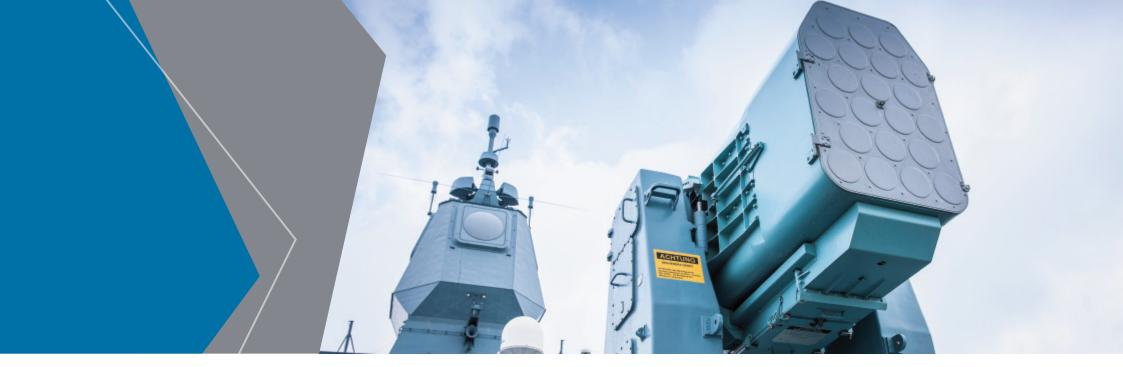
Rolling Airframe Missile (RAM) is fire-and-forget Close-In Weapon System (CIWS) for ship self-defence against Anti Ship Missiles (ASM), helicopters, aircraft and surface targets. RAM was designed to engage the most challenging threats and is the only ASM defense system capable of effectively coping with multiple and high density raids, even in littoral scenarios.
